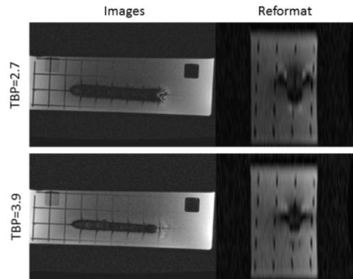
Figure 2. Increasing the refocusing time-bandwidth product (TBP) allows signal near the metallic implant to be recovered at the cost of increased in-plane distortion. Axial images and sagittal reformats show that the acquisition with a TBP=3.9 refocusing pulse has less signal dropout than the TBP=2.7 refocusing pulse; however, the grid lines are more distorted in the frequency encode direction.
