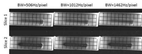
Figure 3. Increasing the receiver bandwidth reduces the in-plane distortions associated with frequency encoding. Images of two slices acquired at different receiver bandwidths and matching refocusing time bandwidths of 3.9 show the grid lines getting less distorted as the receiver bandwidth increases.
