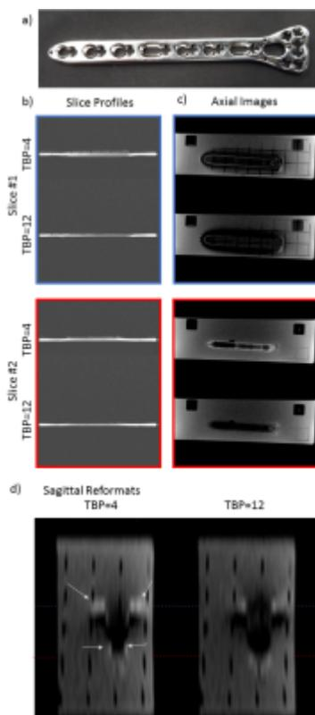
Figure 1. The use of high bandwidth excitation RF pulses reduces through-plane distortions caused by a 316L stainless steel compression plate (a). Slice profiles (b), axial images (c), and sagittal reformats (d), are shown for two slices and two excitation time-bandwidth products. Arrows in the sagittal reformat point to regions of signal pile-up caused by slice distortion which are substantially reduced for higher time-bandwidth product excitation.
