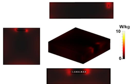
Figure 4. Plots of 10-g local SAR: x-, y-, and z-axis cut-planes are provided through the isocentre of the implant, with an isometric rendering visible in the middle of the figure.
