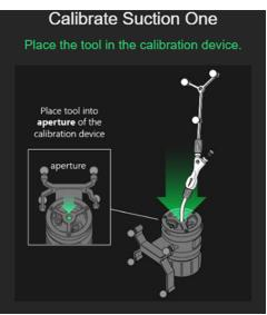
Figure 63 Calibrating a Trackable Suction tool
