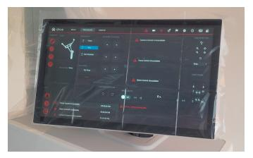
Figure 30 Monitor drape applied to touchscreen monitor
