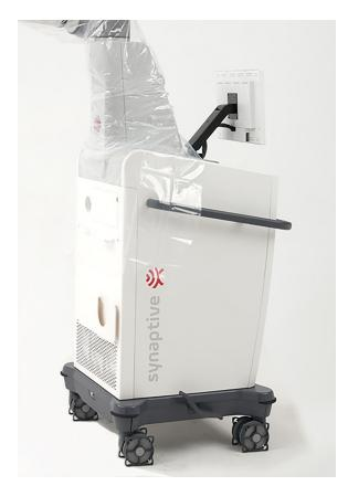
Figure 39 Skirt drape applied around positioning arm base
