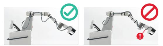
Figure 11 Correct and incorrect cable positions. The red callout indicates incorrect cable positioning wrapped around the end effector.
