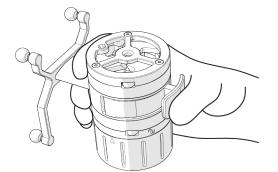
Hold the Calibration Device securely in the palm of your hand with the tracking array between your index and middle fingers.
