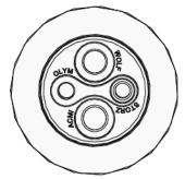
Figure 40 Auxiliary light source connectors
