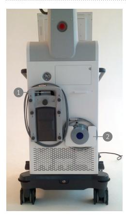
Figure 16 Pedals stowed in mobile base
