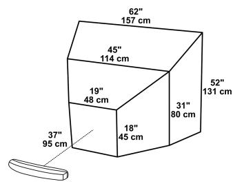
Figure 26 Tracking camera field of view
