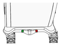
Figure 3 Modus X caster brake pedal
