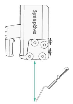
Figure 9 Standoff distance for the Pointer tool
