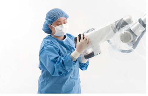
Figure 34 Pressing the marker posts onto the end effector
